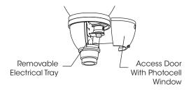
**YD & YE Twist Lock Photocell Fitters**
