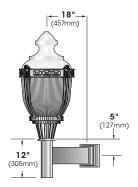
Extruded aluminum arm bracket and cast aluminum wall bracket.
