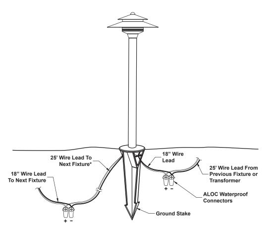
\*Terminate And Cap Leads if Last Fixture On Run
