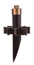
PERMAPOST (PRM) Heavy Duty Mounting Stakefor Deep Anchoring in High Traffic Areas and/or Longer Mounting Stems. 18.5" Long with 3" Dia. PVC Body. 9" Wide Stabilizing Fins and Locking Brass Cap.
