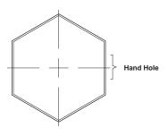
Note: Anchor Plate for Pole Assembly used with this decorative 2-pc Base must fit inside a 25" dia.
