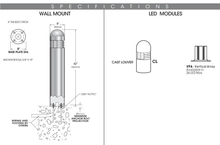
\* When mounting in soil, anchor bolt fasteners and other hardware must be protected from soil by grouting.
