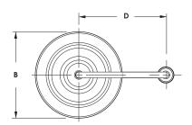
Fitter supplied to fit over 2 <sup>7</sup>/8" X 3" (73mm X 76mm) tennon.
