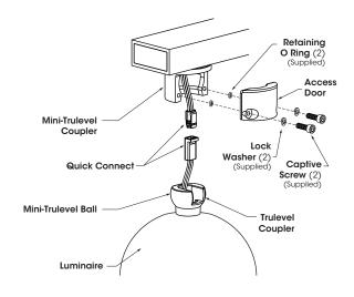
Loosen (2) Captive Screws and remove Access Door from Mini-Trulevel Coupler, pull out Quick Connect from Mini-Trulevel Coupler and Mini-Trulevel Ball.
