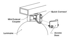
3. Connect Quick Connect components, push components inside of Mini-Trulevel Coupler cavity, replace Access Door and loosely secure, do not tighten.
