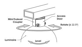
4. Rotate (left to right  $\pm$  22.5°) and level Luminaire to desired position. Tighten Access Door.
