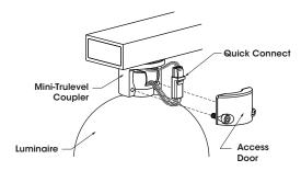
3. Connect Quick Connect components, push components inside of Mini-Trulevel Coupler cavity, replace Access Door and loosely secure, do not tighten.
