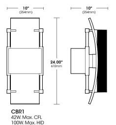
CBR1 (Glare Shield) Corrosion resistant aluminum construction. Shield has tooHess hardware for indexing in one of five (5) positions (1" increments) along vertical Struts.
