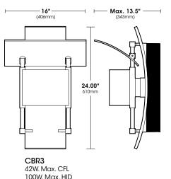
CBR3 (Curved Indirect Reflector) Constructed of corrosion resistant low copper cast aluminum alloy #A356 (<0.2% Cu). Indirect reflector is curved and has stainless steel socket-head screws to secure its vertical position along the Struts. Curved indirect reflector is adjustable for tilt from 0° (horizontal) to 45° up.
