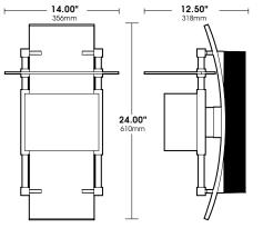
CBR2 (Flat Indirect Reflector) Constructed of corrosion resistant low copper cast aluminum alloy #A356 (<0.2% Cu). Indirect reflector is flat and has stainless steel socket-head screws to secure its vertical position along the Struts.
