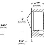
**Baffled Face Models** 70W. Max CFL 150W. Max. HID 18LED Max.
