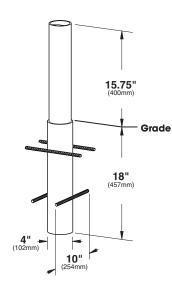
3½" SCH40 STEEL PIPE (below grade) WELDED TO 3"
