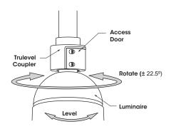
4. Rotate (left to right ± 22.5°) and level Luminaire to desired position. Tighten
