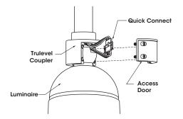
3. Connect Quick Connect components, push components inside of Trulevel Coupler cavity, replace Access Door and loosely secure, do not tighten.
