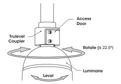
4. Rotate (left to right ± 22.5°) and level Luminaire to desired position. Tighten Access Door
