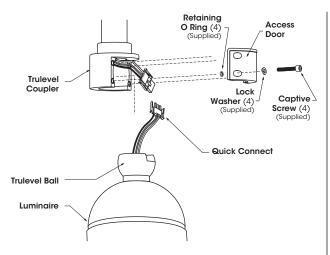
1. Loosen (4) Captive Screws and remove Access Door from Trulevel Coupler, pull out Quick Connect from Trulevel Coupler and Trulevel Ball.
