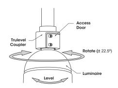
4. Rotate (left to right  $\pm$  22.5°) and level Luminaire to desired position. Tighten Access Door.
