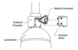
Connect Quick Connect components, push components inside of Trulevel Coupler cavity, replace Access Door and loosely secure, do not tighten.
