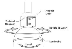
4. Rotate (left to right  $\pm$  22.5°) and level Luminaire to desired position. Tighten Access Door.
