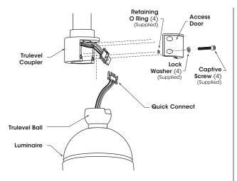
Loosen (4) Captive Screws and remove Access Door from Trulevel Coupler, pull out Quick Connect from Trulevel Coupler and Trulevel Ball.
