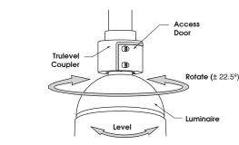
4. Rotate (left to right ± 22.5°) and level Luminaire to desired position. Tighten Access Door
