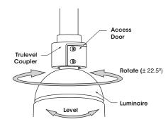
4. Rotate (left to right  $\pm$  22.5°) and level Luminaire to desired position. Tighten
