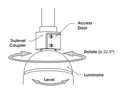
Rotate (left to right ± 22.5°) and level Luminaire to desired position. Tighten Access Door
