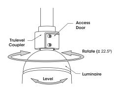
Rotate (left to right ± 22.5°) and level Luminaire to desired position. Tighten Access Door
