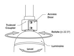
4. Rotate (left to right  $\pm$  22.5°) and level Luminaire to desired position. Tighten
