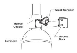
3. Connect Quick Connect components, push components inside of Trulevel Coupler cavity, replace Access Door and loosely secure, do not tighten.
