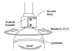
4. Rotate (left to right  $\pm$  22.5°) and level Luminaire to desired position. Tighten Access Door.
