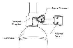
Connect Quick Connect components, push components inside of Trulevel Coupler cavity, replace Access Door and loosely secure, do not tighten.
