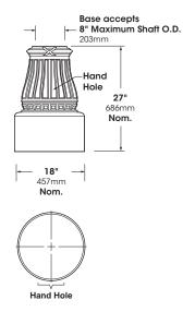
**Note:** Anchor Plate for Pole Assembly used with this decorative 2-pc Base must fit inside a 17" dia.
