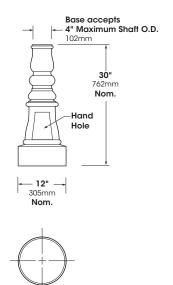
**Note:** Anchor Plate for Pole Assembly used with this decorative 2-pc Base must fit inside a 11" dia.
