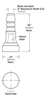
Note: Anchor Plate for Pole Assembly used with this decorative 2-pc Base must fit inside a 13" dia.
