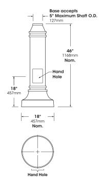
**Note:** Anchor Plate for Pole Assembly used with this decorative 2-pc Base must fit inside a 17" dia.
