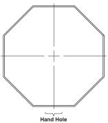
**Note:** Anchor Plate for Pole Assembly used with this decorative 2-pc Base must fit inside a 36" dia.
