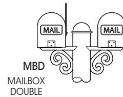
Mailboxes are of durable, corrosion resistant, cast aluminum (A356 alloy; < .02% copper) and painted to match the decorative bollard.
