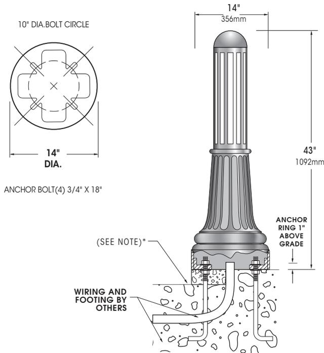
\*When mounting in soil, anchor bolt fasteners and other hardware must be protected from soil by grouting.
