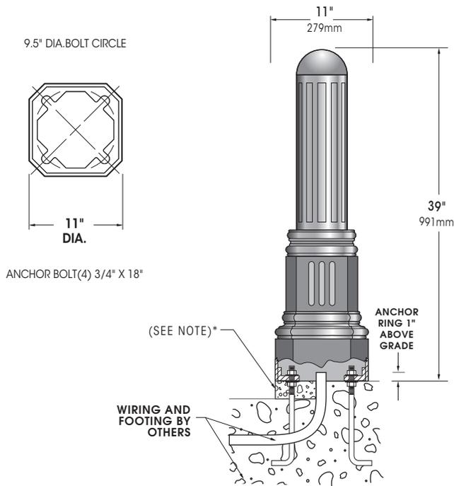
\*When mounting in soil, anchor bolt fasteners and other hardware must be protected from soil by grouting.
