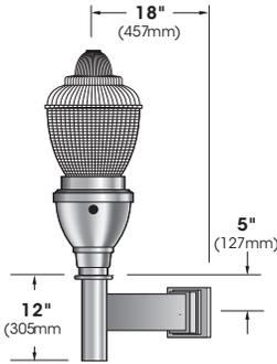
Extruded aluminum arm bracket and cast aluminum wall bracket.
