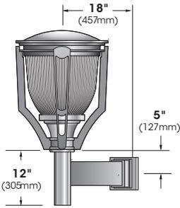
Extruded aluminum arm bracket and cast aluminum wall bracket.
