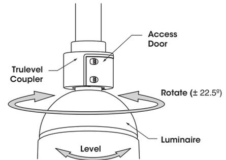
4. Rotate (left to right  $\pm 22.5^\circ$ ) and level Luminaire to desired position. Tighten Access Door.
