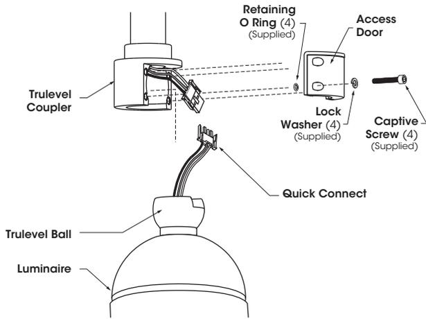
1. Loosen (4) Captive Screws and remove Access Door from Trulevel Coupler, pull out Quick Connect from Trulevel Coupler and Trulevel Ball.
