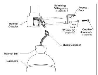
Loosen (4) Captive Screws and remove Access Door from Trulevel Coupler, pull out Quick Connect from Trulevel Coupler and Trulevel Ball.
