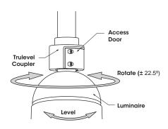
4. Rotate (left to right ± 22.5°) and level Luminaire to desired position. Tighten
