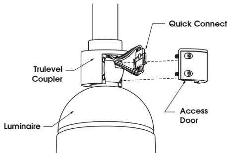
3. Connect Quick Connect components, push components inside of Trulevel Coupler cavity, replace Access Door and loosely secure, do not tighten.
