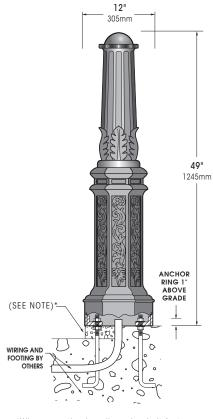
\*When mounting in soil, anchor bolt fasteners and other hardware must be protected from soil by grouting.
