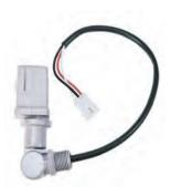
PHOTOCELL Quick Connect Photocell. Swivel Mout with Sliding Adjustment Window. Plugs into Trasformer With Quick Connect Plug. Can be Used in Combination with Timers.
